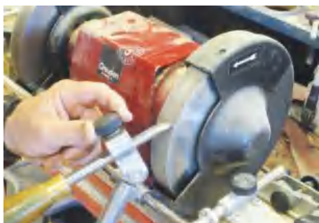
▲ Pic.4 If you find sharpening difficult to master and believe it's not easy to learn, then one of the many grinding jigs available will provide you with a good repeatable shape and sharpness
